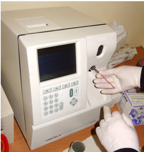
Figure 4: The technical equipment to measure the blood's metabolic data, the so-called Nova Biomedical Phox-M device 19
