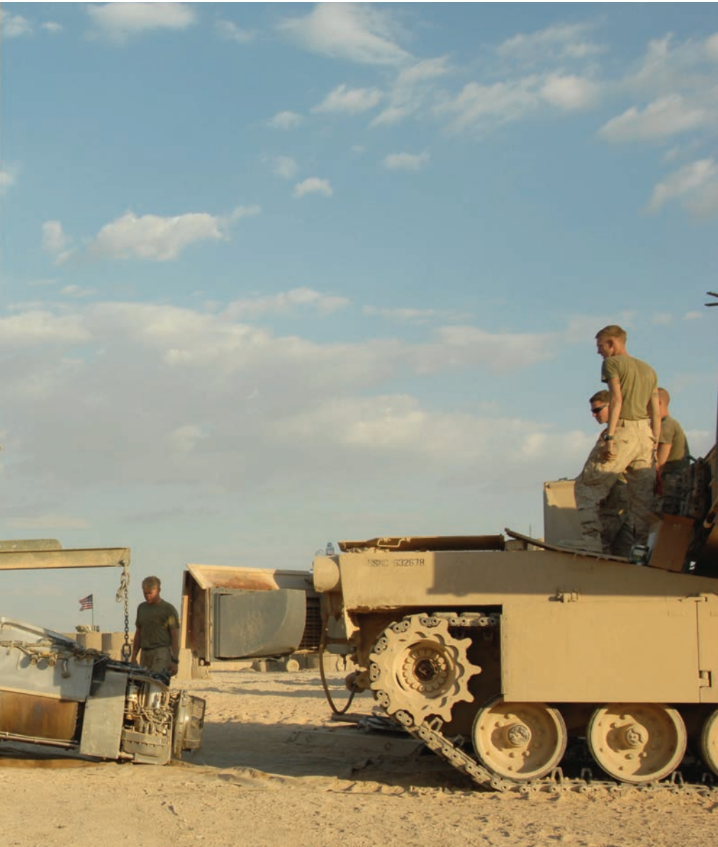
Marines use an M-88-A2 Hercules (left) to repair an M1A1 Abrams tank engine. U.S. Air Force photo by Senior Master Sgt. Dennis Martin.
